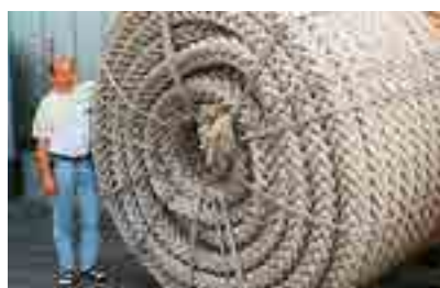
Complete rope cable, total weight approx. 2 t, rope diameter 16 cm
